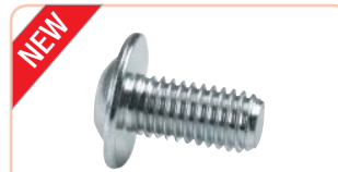
Hex-socket Button Head Screw with Flange ISO 7380-2 10.9 Zinc Plated
