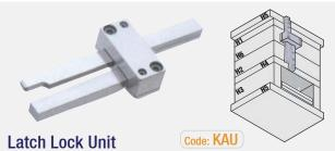
The unit is heat-treated. Safe and reliable with its double sided lock system. It is for two-stage (stripper plate) moulds. The unit can easily mounted due to its compact design. Opening priority of plates relates to the mounting direction of unit. During mounting, after selecting desired stroke, the other Latch Bar is secured.
