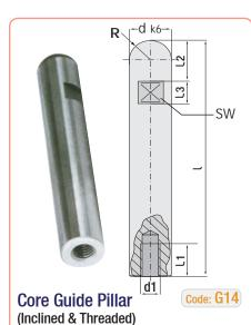
It is compatible to use at injection moulds, angled guide pillar positioning, core systems as cam pin. **GTH** mould pillars are polished with surface polishing machine at final stage of production (after grinding)
