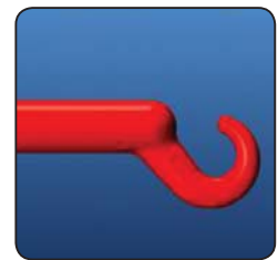
Optimum gate geometry, with edges rounded
