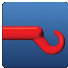
Optimum gate geometry, with edges rounded
