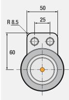
Developed for medium / large moulds. The upper ejector plate stops when reaching the core plate, and the rear plate continues until it reaches the upper plate. As the assembly of the units is not in the center of the mold, but within the ejector frame, the space required for installation is drastically reduced. Double ejection up to 56mm.
