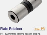
PR - Guarantees that the second opening stays closed until the first is completely open. 50 Kg. opening load required per unit (Minimum of 2 parts required). Possibility to change inner spring from the parting line. Also protects mould affecting from vibrations and impacts by reducing speed tension and absorbing pinking during opening. The most important advantage of it is to extent life time of mould parts.
