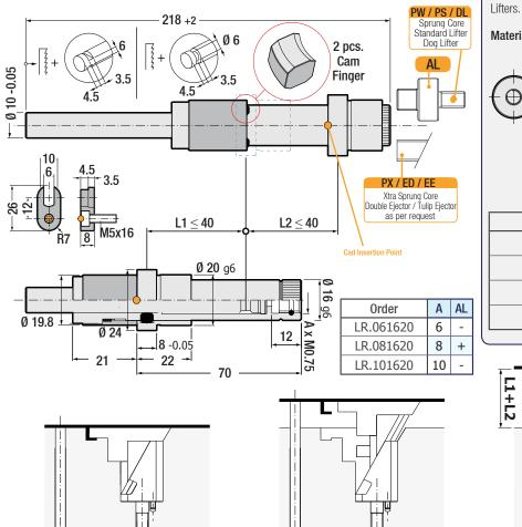
**Threaded Limiter Adapter** Allows the use of the LR for internal threads. It is a dual different threaded adapter providing positioning of LR. In Addition: Fine tread part of AL also can be used as joint adapter for PW - Sprung Cores & PS - Standard Material: 1.5065 8 ± 0.05 80 × M0.7 16 -0.2 ÎВ Œ 6 Adaptable to LR.081620 Code: AL Order В AL.0800M4 M4 x 10 AL.0800M5 M5 x 10 AL.0800M6 M6 x 10 AL.0800M8 M8 x 10 DL Cumsa Dog Lifter L1+L2 **L1**
