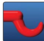
Optimum gate geometry, with edges rounded
