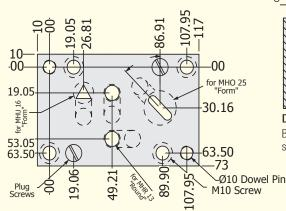
"U" Cut Punch Knock Out Hole **Detail View of Punch Hole**
